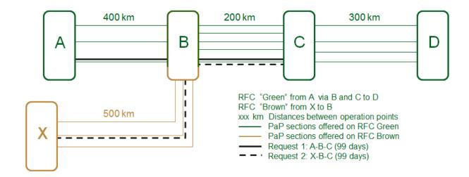
Calculation of priority value:  $K = L_{PAP} \times Y_{RD}$ Request 1:  $K = (400 \text{ km} + 200 \text{ km}) \times 99 \text{ (days)} = 600 \times 99 = 59,400$ Request 2:  $K = (500 \text{ km} + 200 \text{ km}) \times 99 \text{ (days)} = 700 \times 99 = 69,300$
