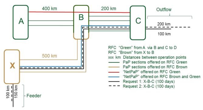
1<sup>st</sup> step calculation of priority value: K = L<sub>NetPAP</sub> x Y<sub>RD</sub>
